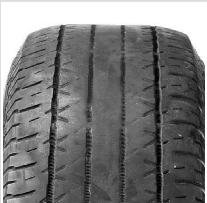
Worn at or below wear bar (legal limit - 2/32")
