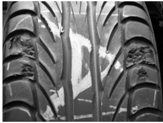
Wheels locked during braking application.
