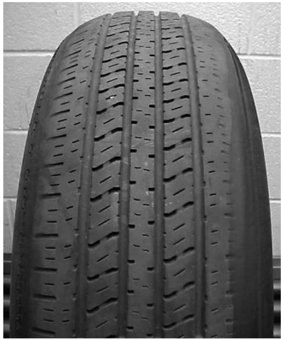
Shoulder wear due to misalignment, mechanical wear or improper tire inflation.
