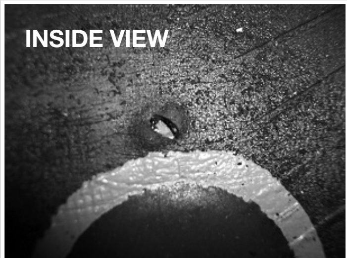
Stone drilling from misapplication or spinning/ driving on unimproved roads.
