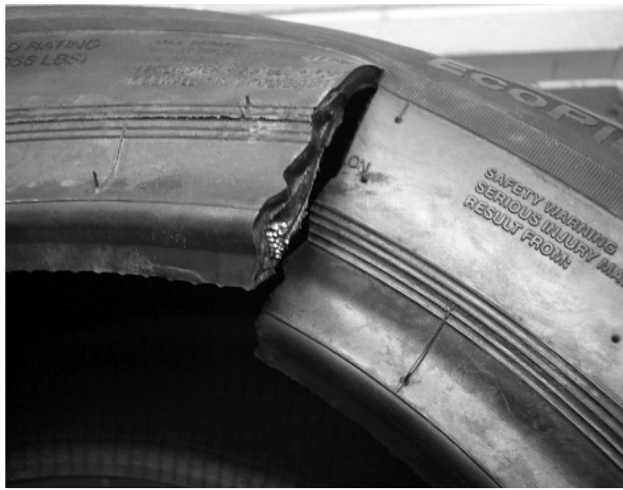
Bead broken due to improper mounting process.
