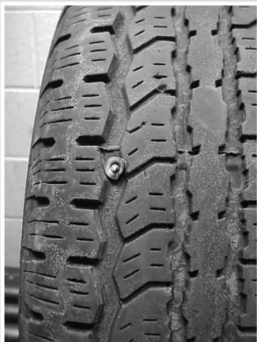
Run Flat due to puncture penetration.
