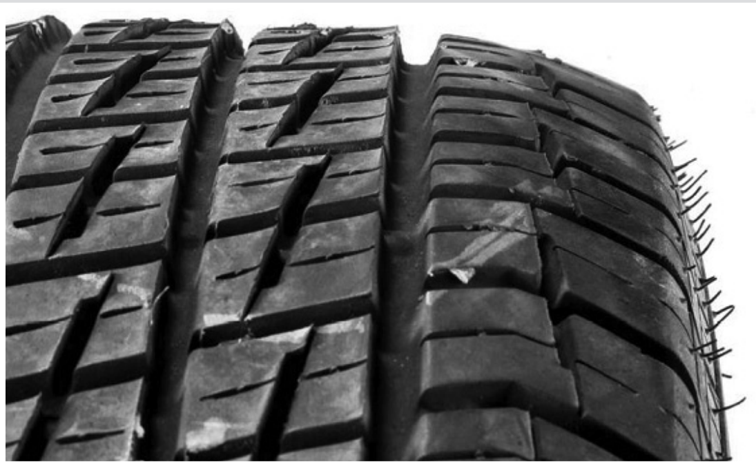
Feathering due to misalignment, mechanical wear or improper tire inflation.
