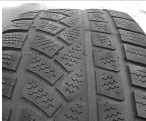
Center wear due to misalignment, mechanical wear or improper tire inflation.
