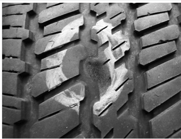
Impact damage to tread.
