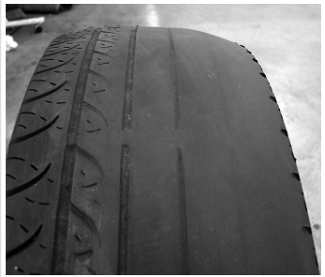
Excessive one-sided wear due to misalignment.
