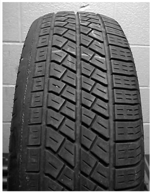
Excessive one-sided wear due to misalignment.
