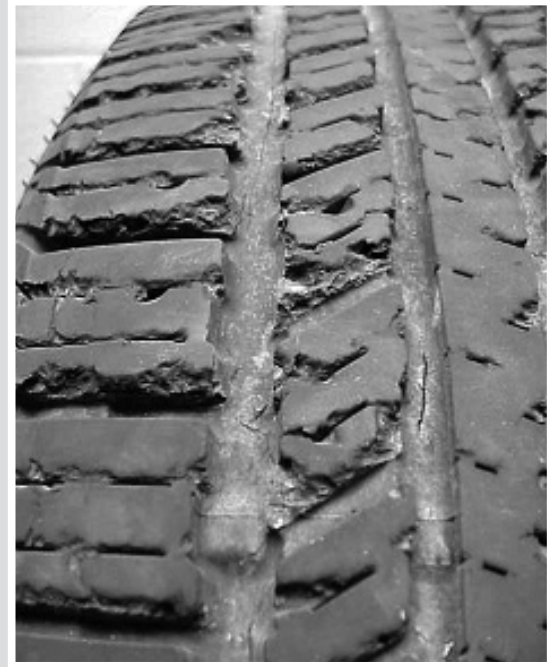
Tread torn or chipped from misapplication or spinning / driving on unimproved roads.
