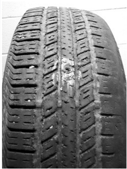
Stone drilling from misapplication or spinning/ driving on unimproved roads.
