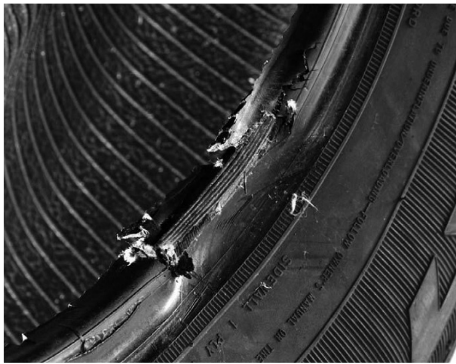
Bead broken due to improper mounting process.
