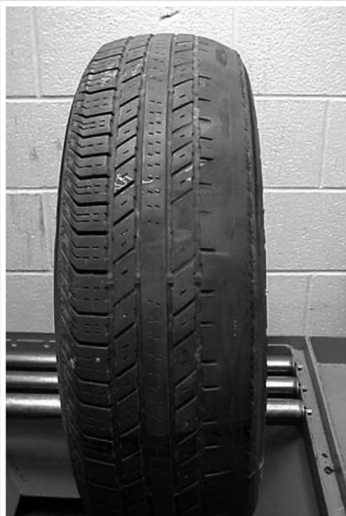
Diagonal wear due to misalignment, mechanical wear or improper tire inflation.
