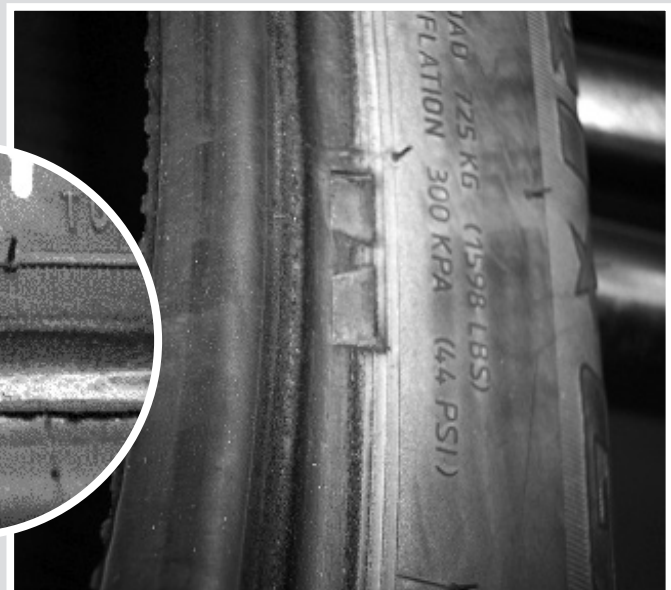
Rim chafing due to underinflation/overload.
