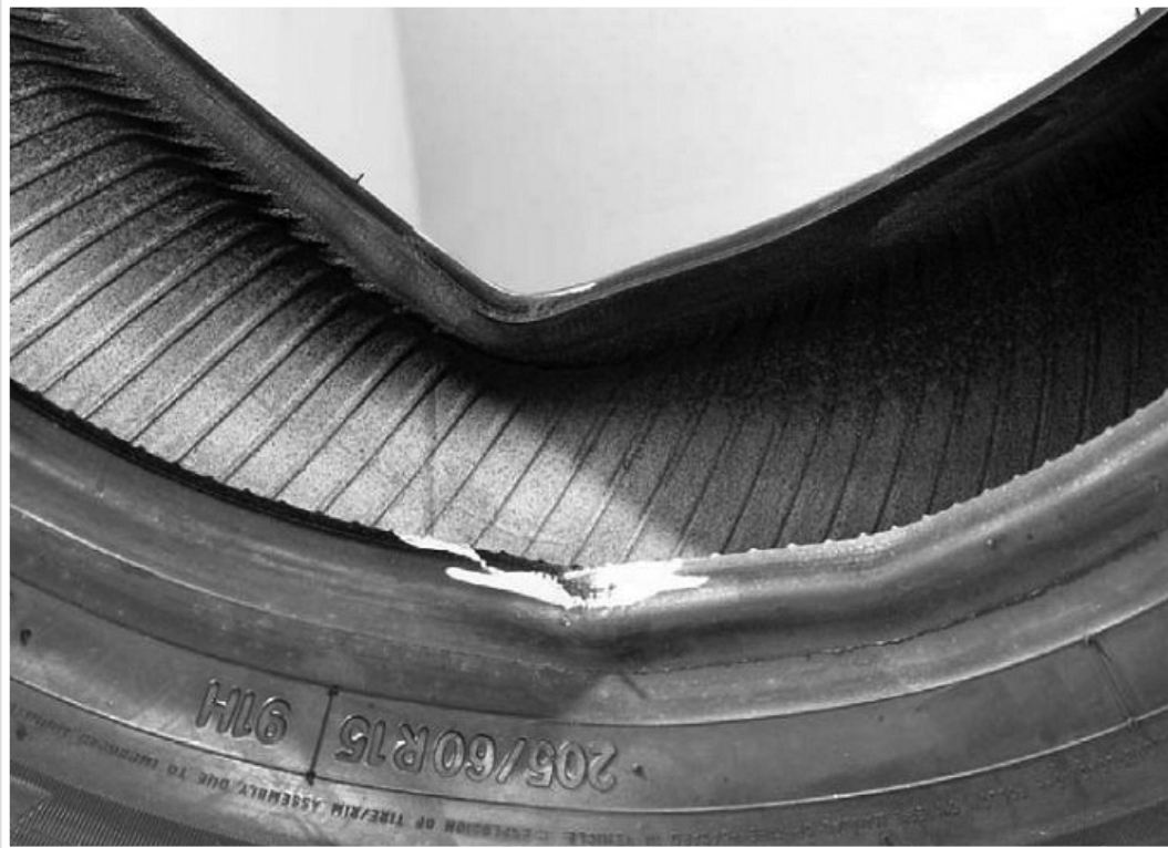
Bead damaged/kinked during mounting.
