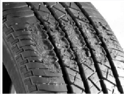
Wheels locked during braking application.
