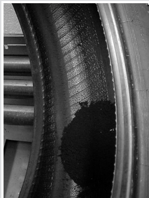
Run Flat due to puncture penetration.
