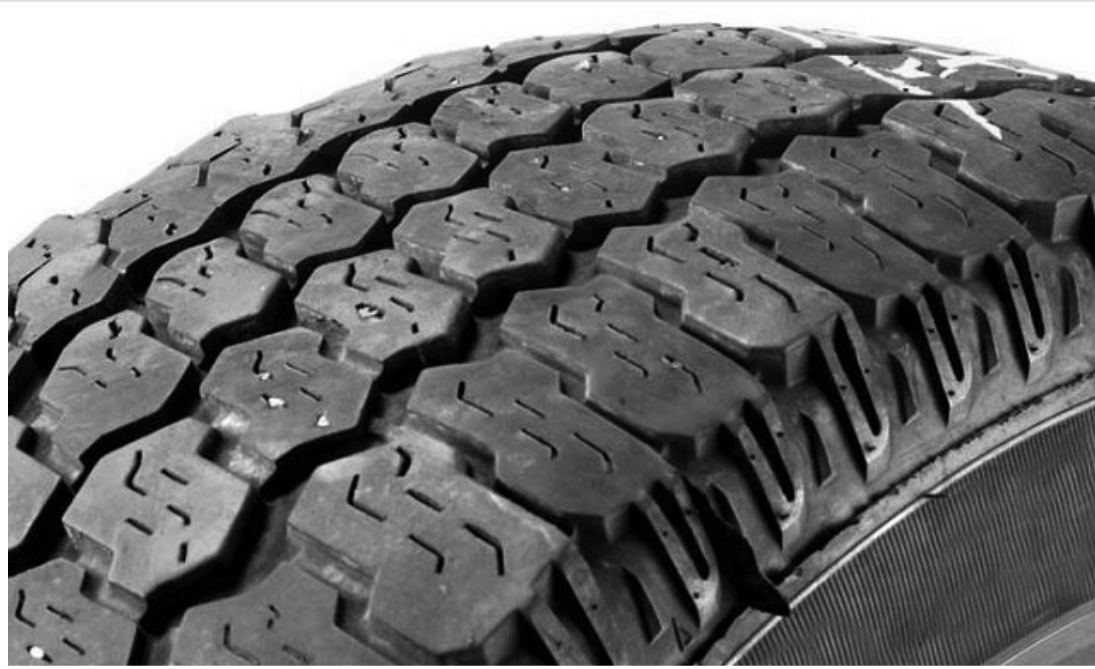
Cupping due to misalignment, mechanical wear or improper tire inflation.
