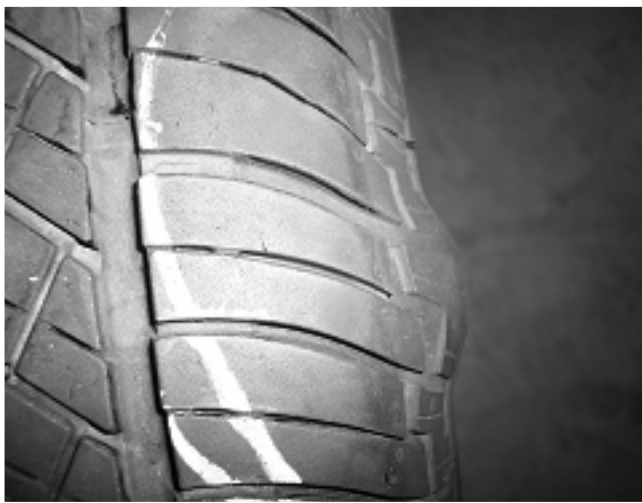
Sidewall bruised/cut by the rim due to hitting a curb, road hazard, or foreign object.
