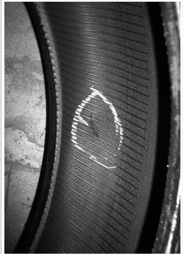
Sidewall bruised/cut by the rim due to hitting a curb, road hazard, or foreign object.
