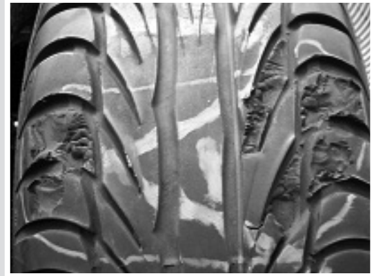
Wheels locked during braking application.
