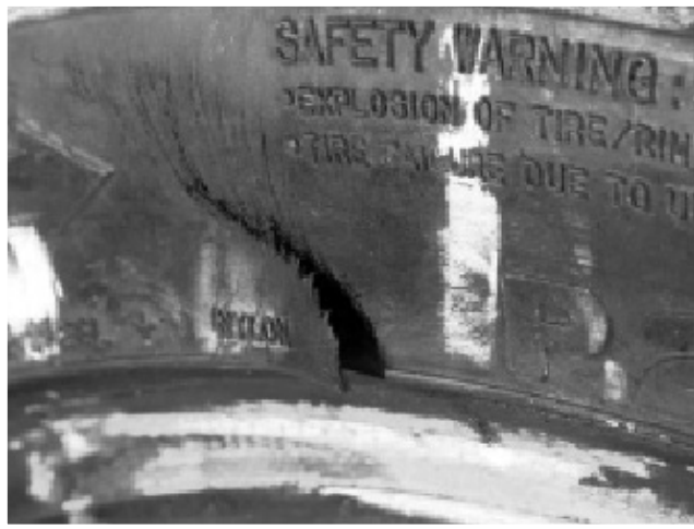
Sidewall cut/snagged due to hitting a curb or debris on the roadway.
