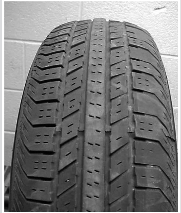
Irregular wear due to misalignment, mechanical wear or improper tire inflation.
